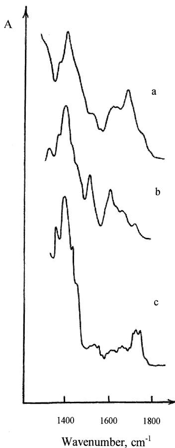
FIGURE 3 IR ATR spectra of the surface of the destroyed adhesion joint. Substrate is SKF-26 rubber: (a) substrate was not roughened before joint formation; (b) substrate was roughened before joint formation; (c) initial SKF-26 substrate surface.
